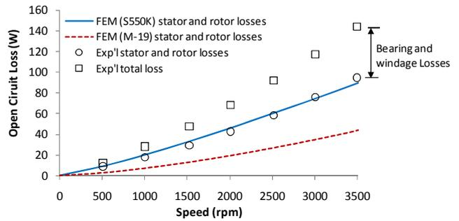
Figure 10: FE and measured open-circuit loss as a function of speed.
