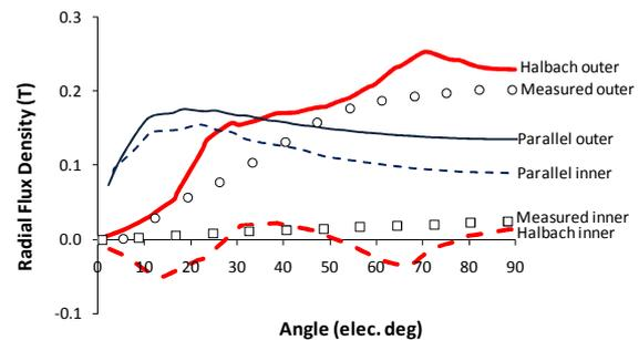
Figure 6: Measured flux density on the surface of bonded-ring magnet in comparison to the FE Halbach 4 segments/pole and parallel magnetization using magnet properties from the manufacturer
