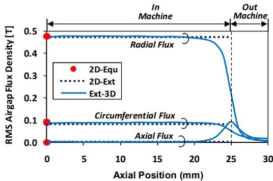
Figure 8: FEM airgap flux densities under open-circuit conditions
