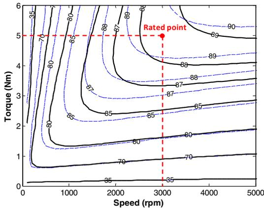
Figure 16: Calculated efficiency map plotted with the measured (solid lines) and FE (dashed lines) back-EMF assuming  $E$  and  $I$  are in phase
