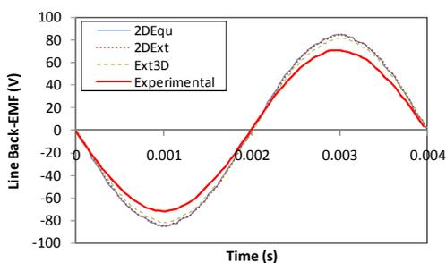
Figure 5: Line back-EMF waveforms at 3,000rpm, comparison of the experimental and the three FE model predictions
