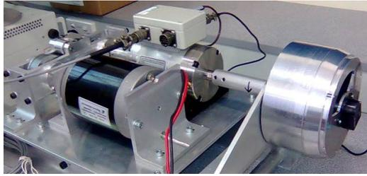
Figure 4: The test rig showing the DC load machine, belt drive, torque transducer and prototype SMC machine (right)
