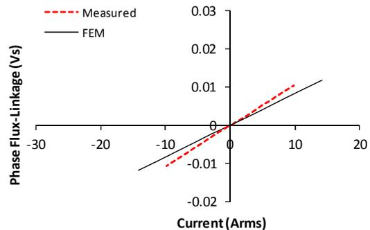
Figure 11: The FE and measured flux-linkage versus current for the case without the rotor in the machine
